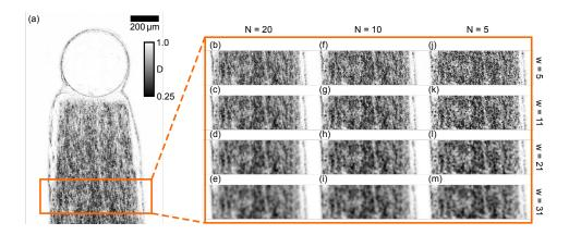
**Figure 4**. (a) Dark-field signal of the sample obtained with N = 20 steps and a window size w = 5. (b)–(m) Dark-field signal in a region of interest in the wooden toothpick reconstructed with different parameters.
