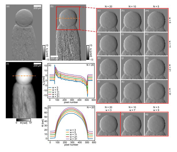
**Figure 3**. Refraction angles in the vertical (a) and horizontal (b) directions for N = 20, w = 5. Panels (c)–(q) show the horizontal refraction of the sphere reconstructed for different window sizes w and numbers of steps N. (r) Phase shift integrated from (a), (b). (s), (t) Line plots through the horizontal refraction and integrated phase in the sphere for N = 20 and different w. Lines are offset by 1.5 µrad in (s) and 4 rad in (t) for clarity.
