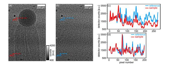
**Figure 2**. Speckle interference patterns with (a) and without (b) the sample in the beam. Panels (c) and (d) show line plots through the patterns at the positions of the sphere and the toothpick, as indicated in (a), (b).
