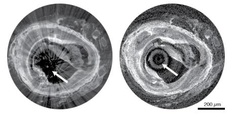
Figure 4. Comparison of phase tomography (left slice) and laboratory  $\mu$ CT (right slice) using a slice that contains an air bubble. The trapped air causes artifacts that prevent the segmentation of the vessel lumen in phase tomography data.
