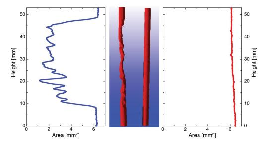
Figure 1. Cross-sectional area of the inner volume of a diseased (left) and healthy (right) artery model derived from laboratory μCT measurements. In the center, the data are represented as 3D rendering.
