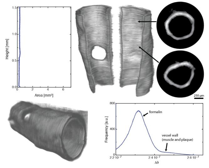
Figure 2: Morphology of a stenosed mouse aorta from a phase SRµCT measurement. Top, left to right: diagram of the cross sectional area of the lumen with axes comparable to the diagrams in Figure 1, 3D rendering of the artery bisected and opened up down the middle, with two selected cross-sectional slices. Bottom left to right: 3D rendering of the entire mouse aorta, histogram of the 3D tomography data to elucidate differences in the real part of the refractive index.
