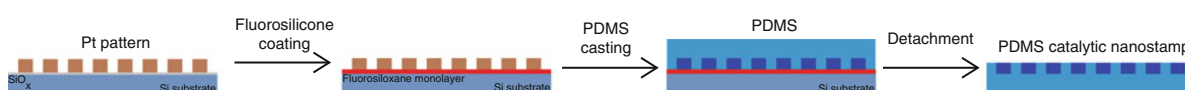
Nanoengineered Hydrogels for Cell Engineering, Fig. 2 Schematic diagram for fabrication of PDMS nanostamp (Ref. [8])
