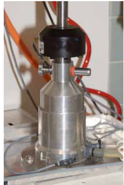
The team of Bert Müller uses this device to simulate coughing and to test the adaptability of the artificial sphincters.
