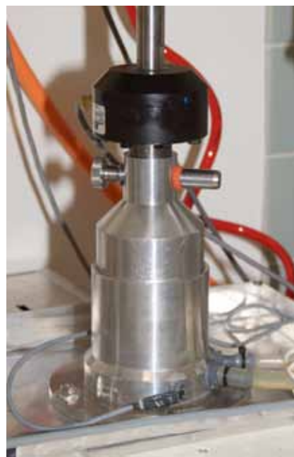
The team of Bert Müller uses this device to simulate coughing and to test the adaptability of the artificial sphincters.
